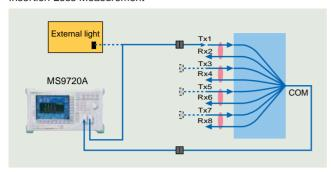
By using the same setup, it is possible to measure the optical leakage between each channel of an optical coupler and to measure the isolation. Moreover, when used in combination with an external light source, it is possible to measure the directivity to evaluate the very weak optical leakage between send and receive channels.
