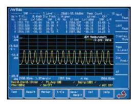
The screen below shows analysis of a 16-channel WDM waveform; the level difference of each channel is displayed using the channel on the left side as a reference. Any channel can be set as the reference.
