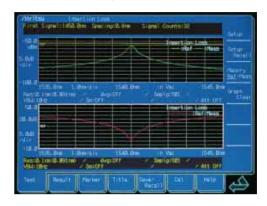
In addition, the measurement results for a specified WDM channel wavelength can be displayed as a list.
