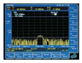
The SNR is improved by using averaging processing. The following is an example of measurement result after 10 sweep averaging are performed.
