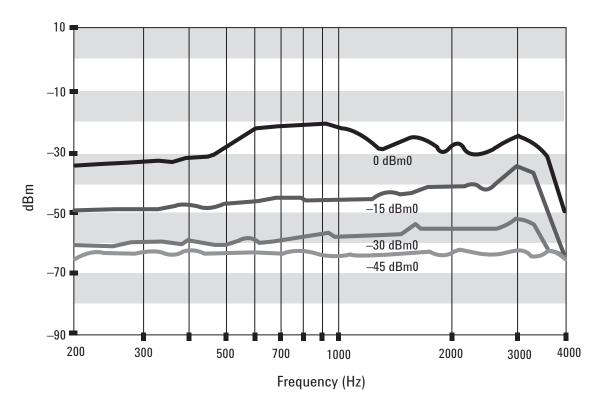
Figure 2b. CVSD distortion dBm characteristic
