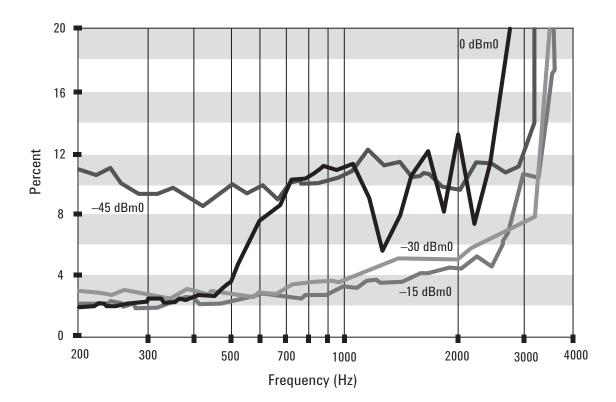
Figure 2a. CVSD distortion percentage characteristic
